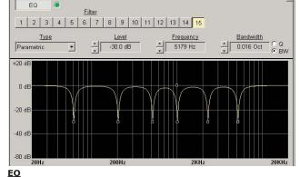
15 Total - Choose from parametric, shelf or allpass. Adjust frequency, level and O
